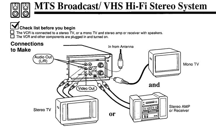
When recording, you may monitor in stereo, by connecting the VCR to either a stereo TV, or a mono sound TV with stereo amp and speakers.
