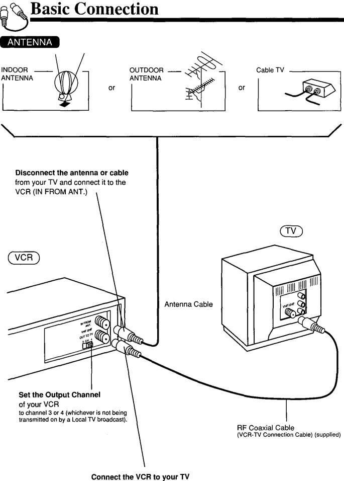
with the RF Coaxial Cable (OUT TO TV).
