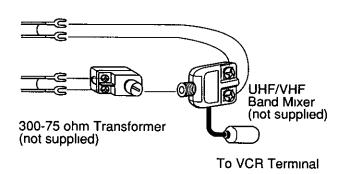
If your TV has both post and screw-type VHF terminals, using the post connection is recommended to minimize signal loss
